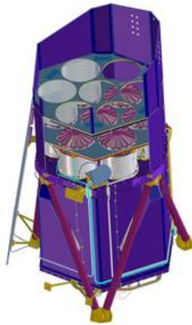
Figure 4.1 The eROSITA telescope will survey sources in and beyond our galaxy in the X-ray spectrum. CAD model from Predehl (2010).
