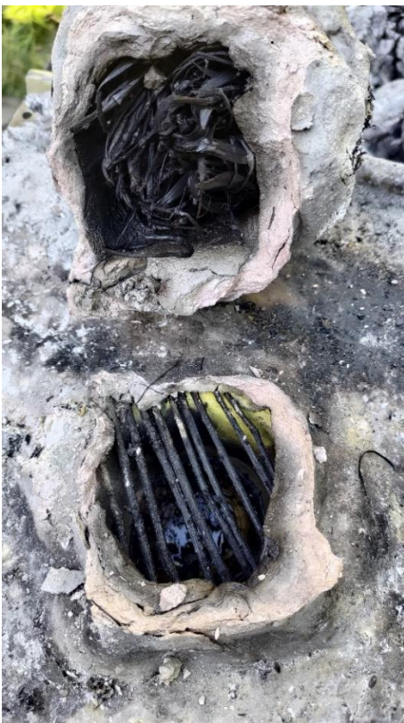
A second way to produce tar from Podocarpus is dry distillation of the leaves using an underground distillation apparatus like this one, which was opened here after the experiment. Photo: Tabea Koch
