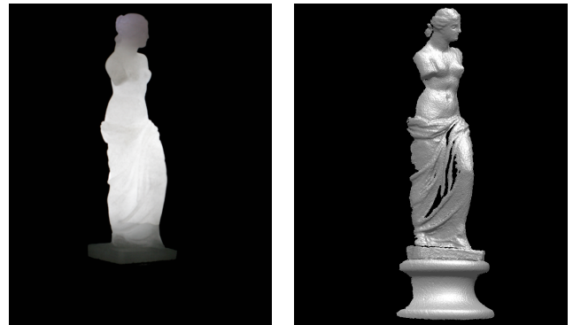
Figure 1. By combining phase-shifting and polarization our method faithfully captures the 3D geometry of very translucent objects such as this alabaster Venus figurine (height \approx 19cm).
