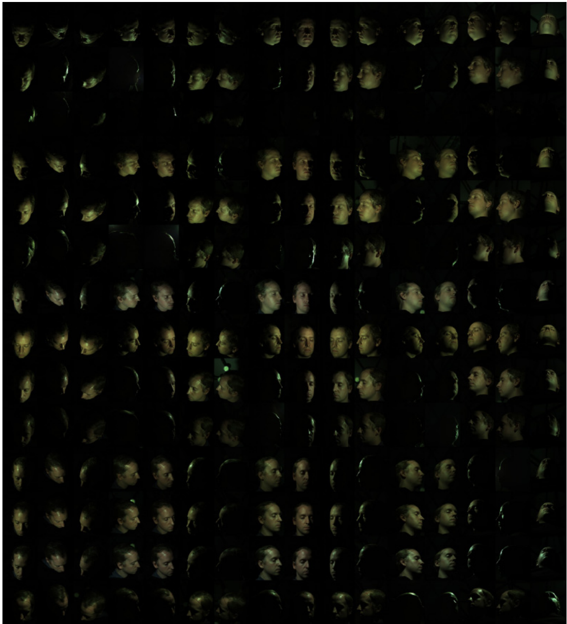
Figure 5.2: Raw reflectance images of a subject acquired with all 16 cameras and 14 (of 150) lighting conditions. Each row shows images with different camera viewpoints and the same lighting condition. Each column displays images with different lighting conditions and the same viewpoint. The images are not yet color corrected, revealing differences between camera characteristics and light source colors.
