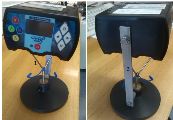
Figure 4.5: Pictures of the hand reflectometer, with the pipes containing the glass fibers (1) and the additional supporting.
