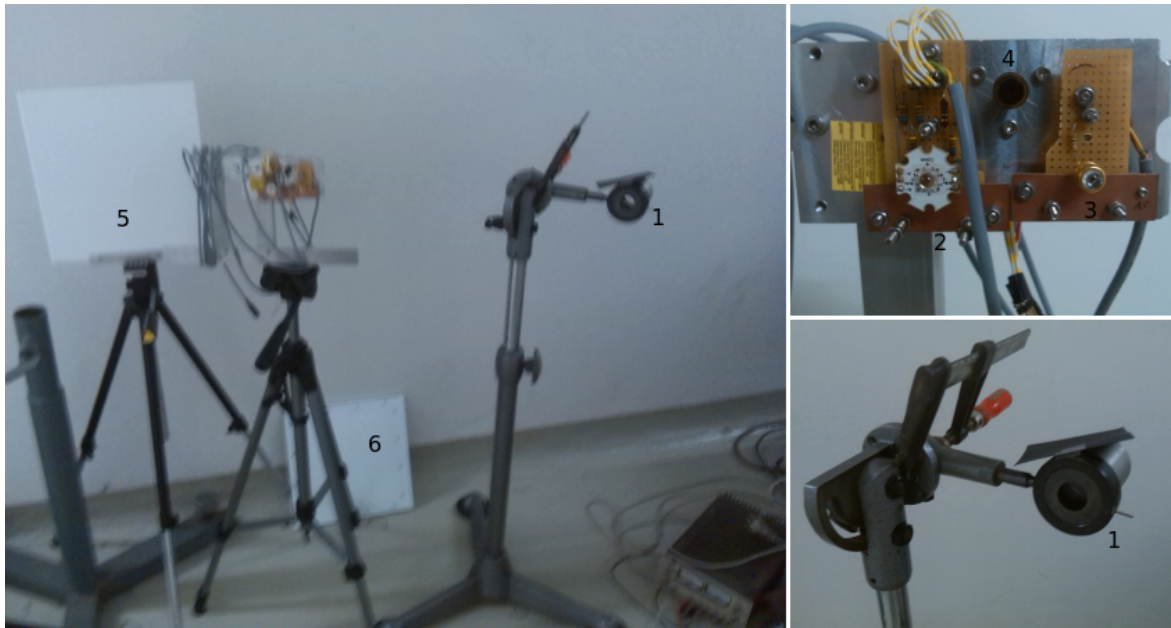
Figure 5.8: Pictures of the components of the new mirror testing setup. 1: The tube with the iris that is positioned before the LEDs. 2: The 4-color-LED. 3: The UV-Led. 4: A laser. 5: The mounted and used Teflon screen. 6: The upgraded Teflon screen. Not in the picture: The Camera.
