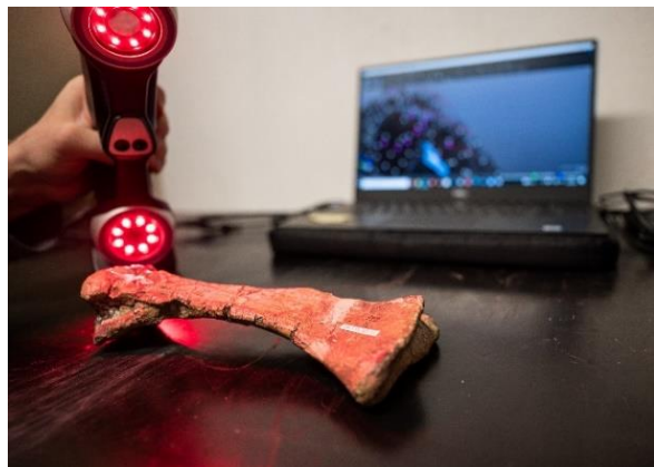
5. 3D image of a footbone from Tuebingosaurus being made with a handheld laser scanner. The colored base with reflective points (left) provides a spatial reference system for the software. Photo: Valentin Marquardt/University of Tübingen
