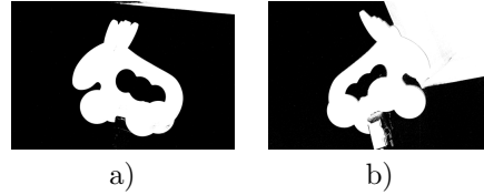
Figure 3. Large regions of wrongly segmented pixels apart from the silhouette (a) and penetrating the silhouette (b).
