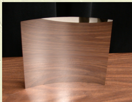
Slumped Glass 5" HEW ~270 kg/m 2
