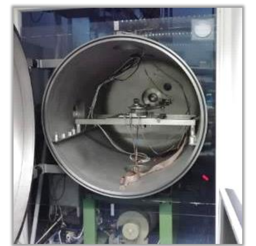
Monochromator setup for FUV QE measurement
