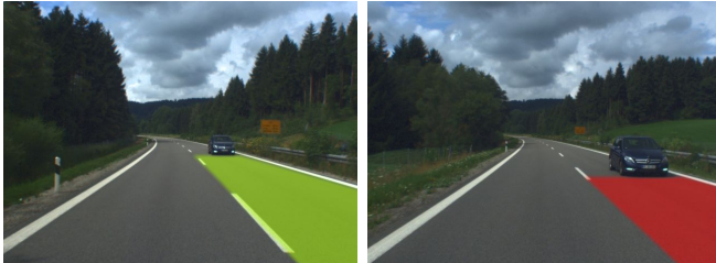
Fig. 5. Time to impact dependent color encoded lane overlay to intuitively visualize the risk potential of a lane change to the driver
