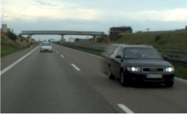
Fig. 8. Artificial exaggerated motion blur, supporting the driver’s assessment of the approaching speed of the trailing vehicle
