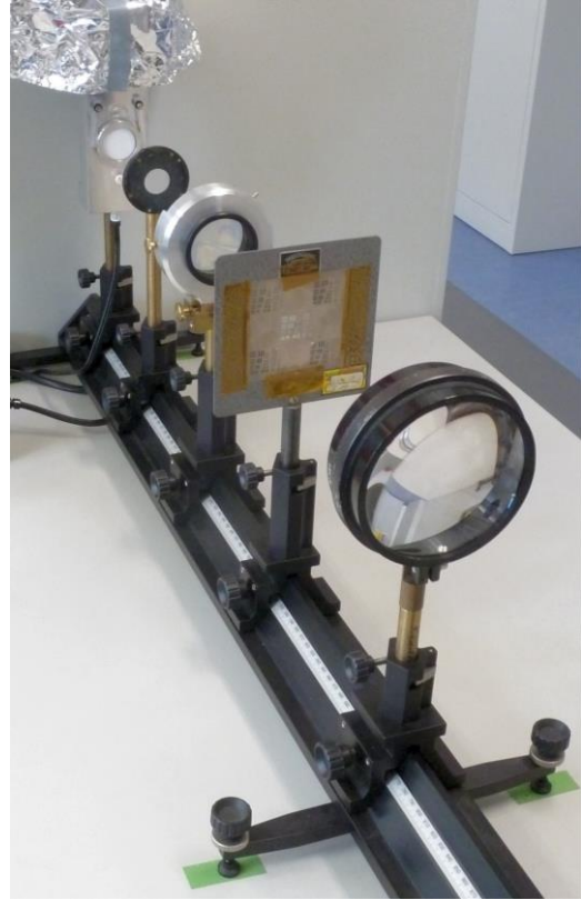
Fig. 3.2 Optical bench with all components (from back to front): lamp, small iris diaphragm, lens with large diaphragm, test mask, condenser lens.
