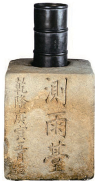
Figure 14: Rain gauge pedestal with a restored rain gauge of the Gyeongsang-do Provincial Office in Daegu (Korean National Treasure No. 330), crafted in the Gengyin year of Qianlong’s reign (1770) (picture by Koh Gyeongmin, https://fr.wikipedia.org/wiki/Cheugugi ).
