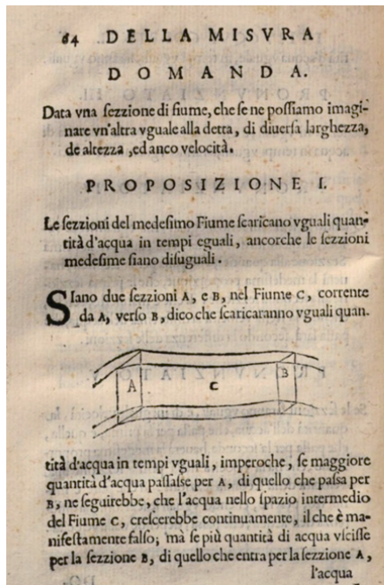
Figure 6: Propos. I of “ Demostrazioni geometriche ”: Sections of a river that carry equal quantities of water in equal times although these sections are unequal (Castelli 1660, Della misura dell'acque correnti , 64).
