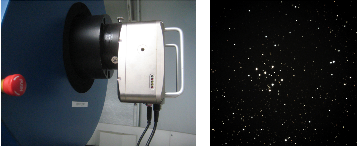
Figure 32: The SBIG STL1001 photometric CCD camera at the left focus of the 80 cm telescope (left). Open star cluster as an observation object for the photometric experiment (right).
