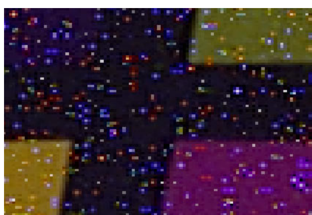
Figure 3: A 422 \times 281 excerpt from an image of a GretagMacBeth ColorChecker taken with the DCS 560 at a film speed of 80 ASA with 25 s exposure time. The image shows four constant colored patches separated by a black cross. The noise is mainly due to “hot pixels” on the CCD chip.
