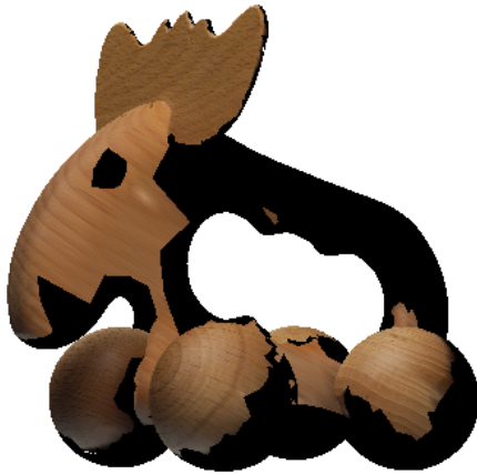
Figure 5: Image of a wooden elk. After registering it with the 3D model of the elk a novel view is rendered. Parts of the model for which no image information is available are shown in black.
