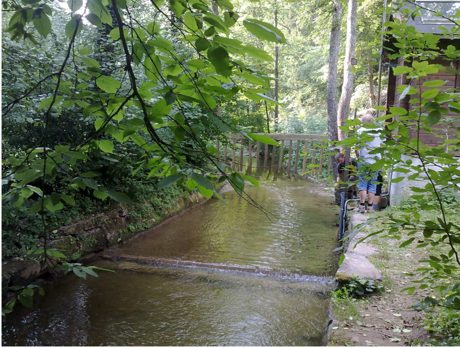
Figure 2.9: A measurement station utilized by WESS group. The small control structure is visible in the river. The goal of the small step is to detach downstream from the upstream to acquire a precise reading on the depth, which is turned into total discharge. Total discharge is used here to provide a calibrated catchment.
