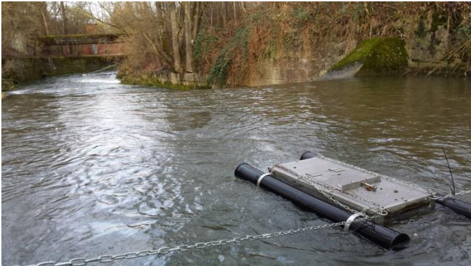
The researchers kept rainbow trout in a special cage in the waters they were analyzing. Photo: Rita Triebkorn
