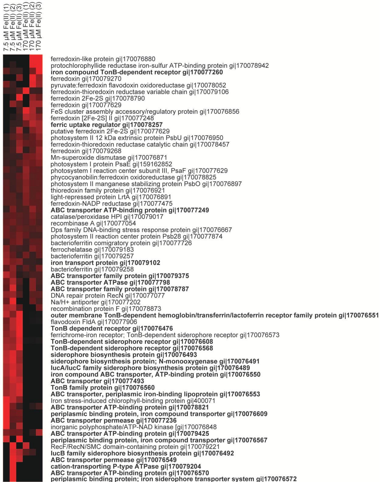
FIGURE 3 | Heatmaps of protein abundance from triplicated biological treatments with low Fe (left columns) vs. when high Fe (right columns) was supplied to Synechococcus PCC 7002 during growth. Each protein was normalized to the average spectral abundance of that protein across all experiments. Red indicates more abundant, black is lower abundance. Proteins in bold are involved in Fe uptake or siderophore biosynthesis and/or import/export. Accession numbers are given for each protein.
