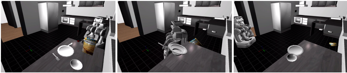
Figure 5. The kitchen robot scenario in the simulated apartment. Left: A simulated PR2 robot starts navigating away from the table. Middle: The robot inadvertently hits the table causing objects to fall to the ground. Right: The robot looks back, detecting more objects lying on the ground.
