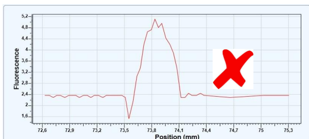
Figure 3.1: Fluorescence signal too low. Increase the LED power or concentration of labeled molecule.
