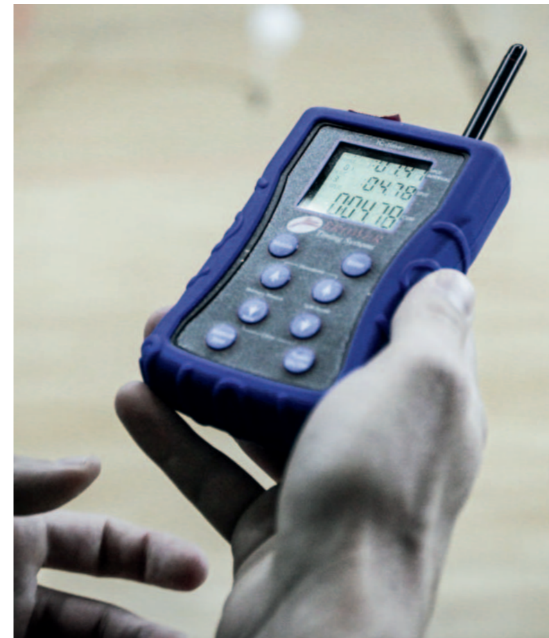
Infrared light barriers transfer the recorded times to the measuring device.
