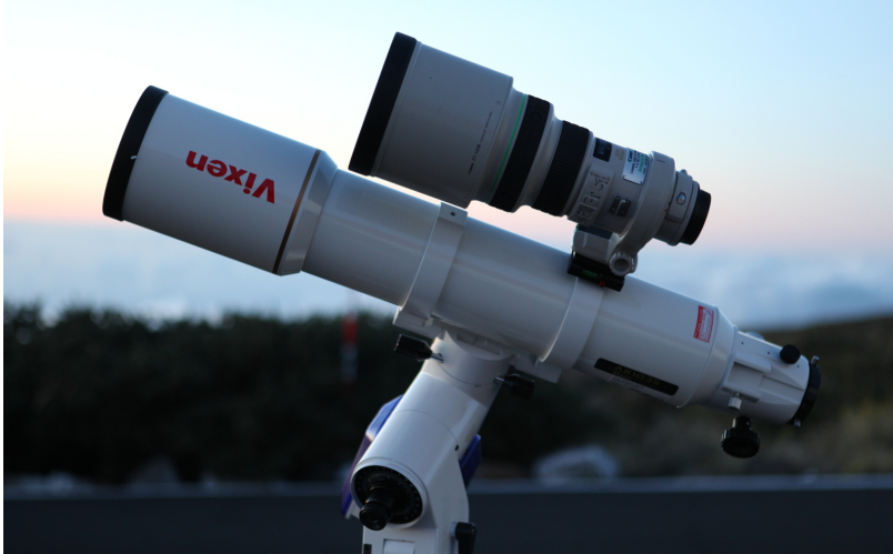
Figure 41: Telescope setup with main and guiding telescope. The guiding telescope is mounted “piggyback” on the main imaging telescope. The cameras are not yet attached.
