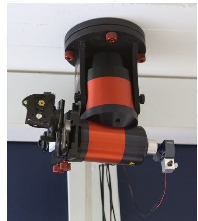
Figure 36: The gearless ASA DDM60 Pro telescope mount, attached to the ceiling of our laboratory.
