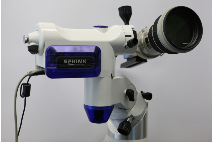
Figure 34: The telescope mount used for the tracking experiments. On the right side is the camera lens used as guiding telescope. A main telescope is not used for the tests.
