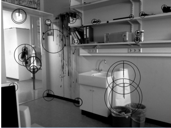
Figure 6. Features detected in a scene are marked by a black circle. The black line in the circle shows the feature's orientation, which is the same for every feature, as the orientation calculation step is skipped.
