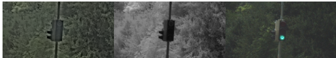
(b) The green lamp of an LED traffic light is not perceived by the NIR channel and is therefore not colorized.
