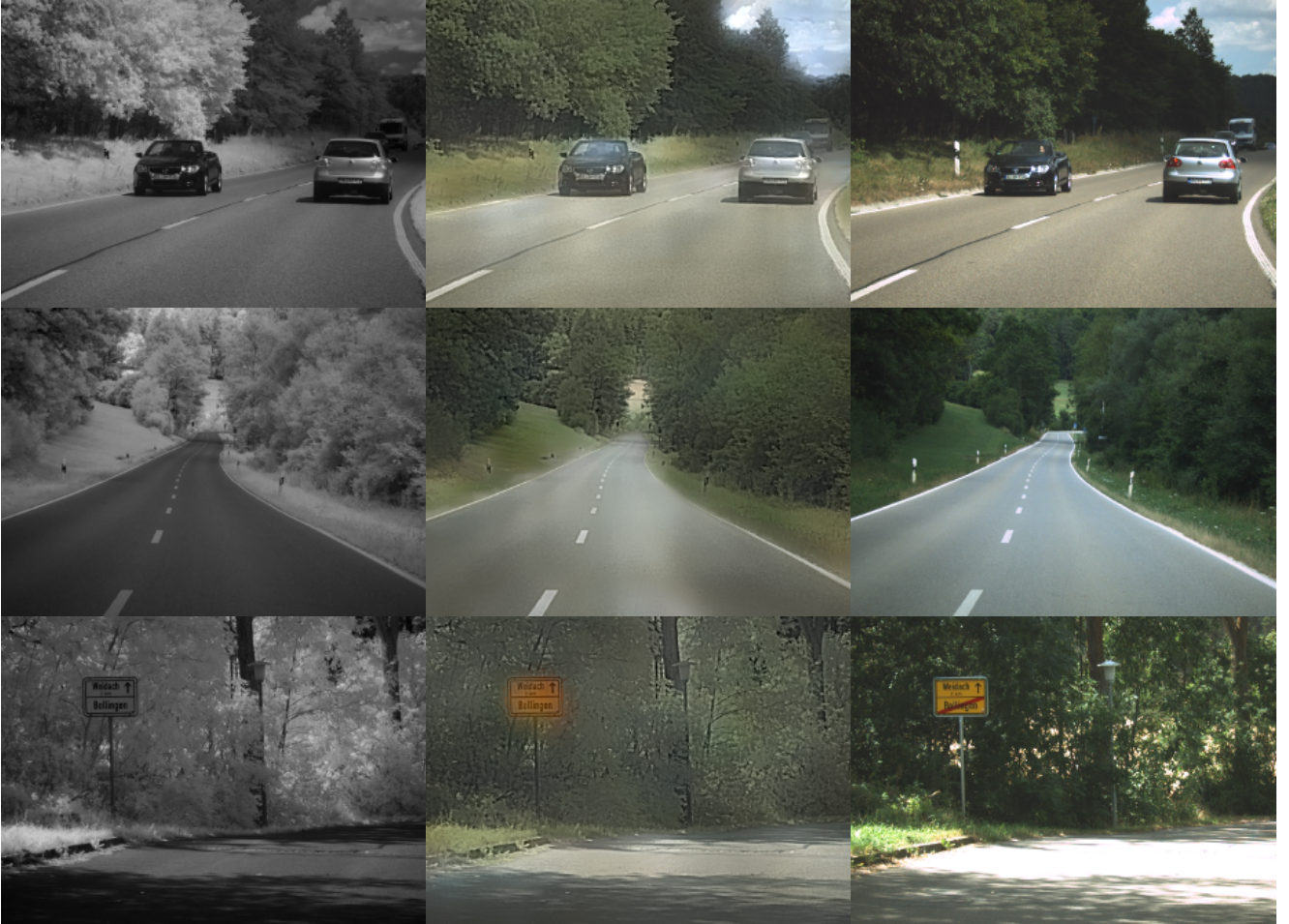
Fig. 10: NIR images (Left) are colored (Middle) in comparison to their target images (Right). The used topology is topo-3-12-3-bp with \sigma_g = 17 and \sigma_f = 0.005 .
