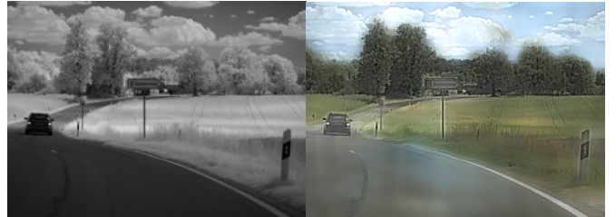
Fig. 1: An NIR image (Left) is colorized (Right) by the approach described in this paper. Best viewed in color.
