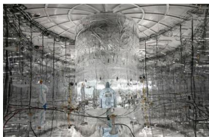
Inside the water tank shielding the GERDA experiment from outside radiation. Tübingen students and researchers have installed photosensors inside this mirrored tank which alert scientists to cosmic rays. Photo: Kai Freund, University of Tübingen
