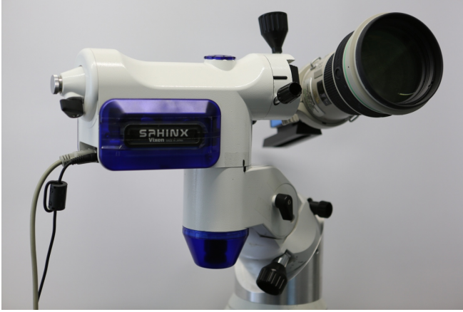
Fig. 6. The telescope mount used for the tracking experiments. On the right side is the camera lens used as guiding telescope. A main telescope is not used for the tests.
