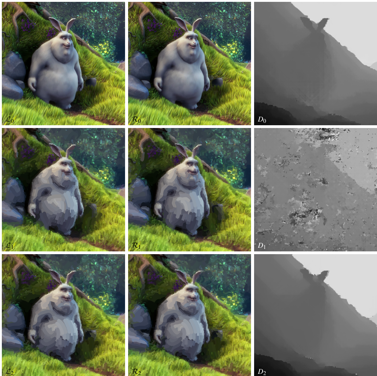
Figure 5: \mathcal{L} and \mathcal{R} from a stereoscopic frame are displayed on the left and an according disparity map on the right. From top to bottom: Original image; SBR without stereo consistency; SBR with our consistency approach. One might notice the different stroke meshes in \mathcal{L}_1 and \mathcal{R}_1 , especially on the bunnys torso. However, in \mathcal{L}_2 and \mathcal{R}_2 they are identical, which again leads to a valid disparity estimation D_2 . Source images : [GR08]
