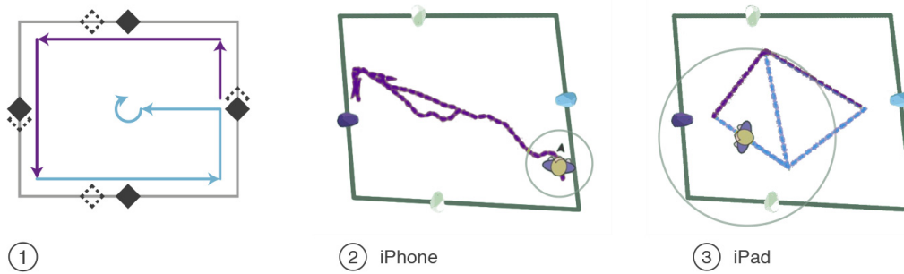
Fig. 1 Localization results with Estimote Indoor SDK. (2) and (3) show the detected trajectory displayed by the Estimote app. The colouring shows two phases of the trajectory; the iPhone only detected the purple part before losing the signal.
