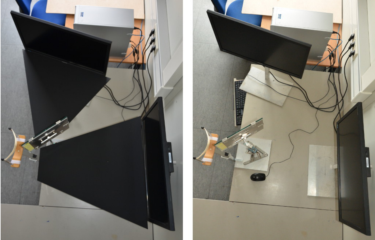
Figure 2.3.: View on the stereoscope from above. In the left image the bottoms of the viewing chamber bottoms are visible. The frontal viewing tunnel has a symmetrical trapeze shaped panel 18.7 cm at the observer's end, and 70 cm side length on the remaining edges. The left panel was an asymmetrical construction of 75 cm, 70 cm, 50 cm, and 20.6 cm with the following angles in the order of the listed lengths: 57^\circ , 72^\circ , 156^\circ , and 74^\circ . The right image shows the plain setup of the monitors and the mirror.
