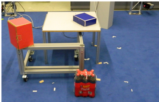
Fig. 1 Movable and static props. Box on the left resembles the form of the actual object. Box on the right does not resemble the form of the actual object. Soda six-pack at the bottom. Table represents the trunk surface. Aluminium structure represents the position of the bumper.
