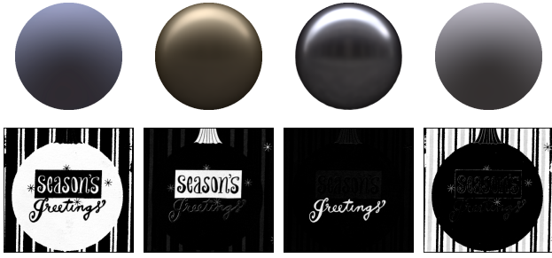
Figure 4: We use a factored representation for svBRDFs, in which each pixel is represented as a linear combination (visualized using the weight maps in the bottom row) of basis BRDFs (visualized in the top row as spheres rendered in the “Uffizi” environment).
