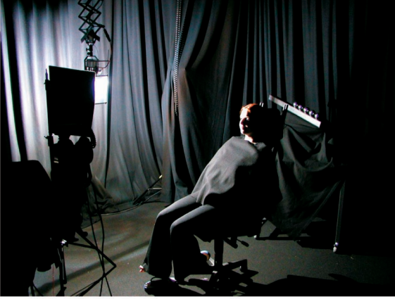
Fig. 2. The measurement setup. The camera (on the left) remains at the same position, while the orientation of the subject’s face and the position of the light source (which is behind a protective pane) are varied. The steel spheres behind the subject are used for measuring the position of the light source relative to the camera.
