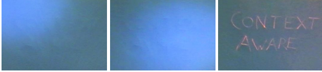
Figure 7. Accumulation of features. Two frames are shown from different grazing light angles with standard illumination. The features of the letters is only faintly visible. In the accumulation mode, features are remembered as the user sweeps the proxy light. This allows us to show all the features at once, making the text visible.
