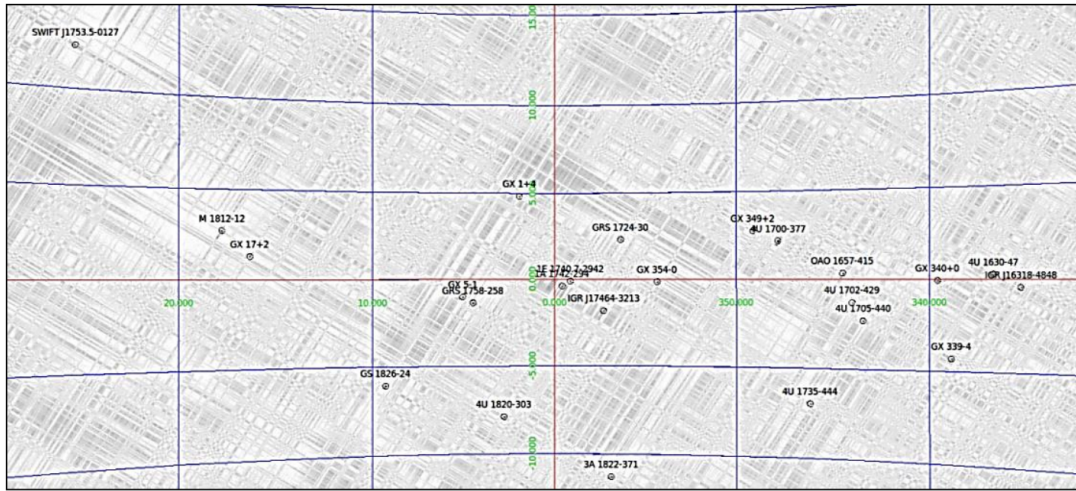
Figure 3.8: Simulated observation of the galactic center with an exposure time of 10 ks. The overlay of the rotated cameras' images causes the stripe structure of the resulting image. Image: LOFT Design Description
