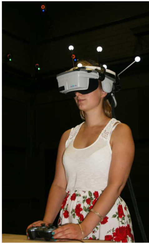
FIGURE 1 | A participant equipped with a head mounted display whose orientation was tracked by motion tracking cameras. Participants used a joystick fixated to a table to adjust their distance estimates.
