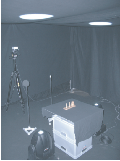
Fig. 1. Photograph of our measurement setup. Spotlight projectors on the floor shine on a tent made from black cloth, and the bounce light illuminates the scene which is arranged on top of the boxes. A tripod-mounted camera records the scene and is protected against lens flares by occluders.
