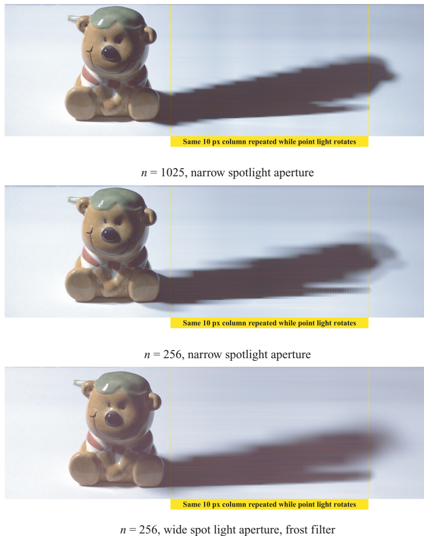
Fig. 4. Results of relighting in point light conditions. Between the two yellow lines, the same vertical strip of 10 pixels width is rendered repeatedly, while the point light is rotated around the up axis over 60 degrees with 0.5 degrees separation. Note the differences between the images at the shadow boundary. For the narrow aperture, n = 1025 images deliver an almost smooth boundary, for n = 256 images, the boundary is strongly jagged, and several overlapping shadow regions can be seen to the right of the image. For the same number of input images and for the same incoming light directions but for full aperture and activated frost filter, the jaggedness is almost not perceivable, and, although the shadow to the right of the image is noticeably blurred, it shows a continuous penumbra zone without ghosting artifacts.
