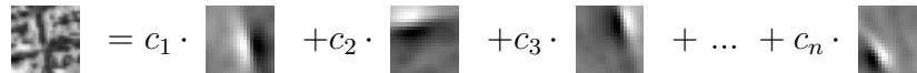
Figure 1.11.: Linear superposition model. An image is represented as a linear combination of several basis images.
