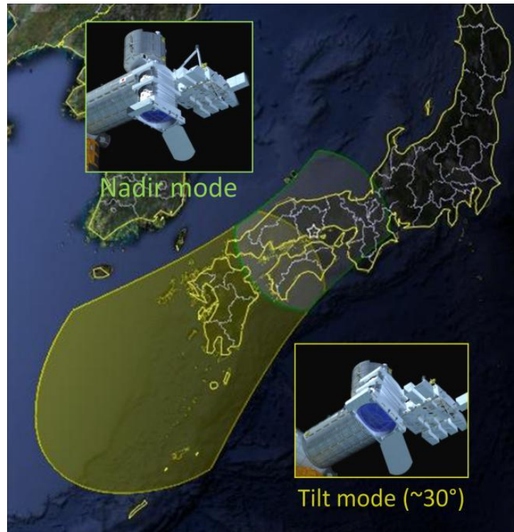
Figure 1.2: Artistic illustration of JEM-EUSO's viewing area: The nadir mode is shown in green and the tilted mode in yellow. A map of Japan is overlaid by the viewing areas. (Image: JEM-EUSO Collaboration, 2010)
