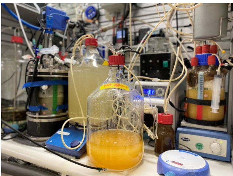
The two-step bioreactor system which was used to produce yeasts enriched with proteins and vitamin B 9 . Photo: Lisa Marie Schmitz
