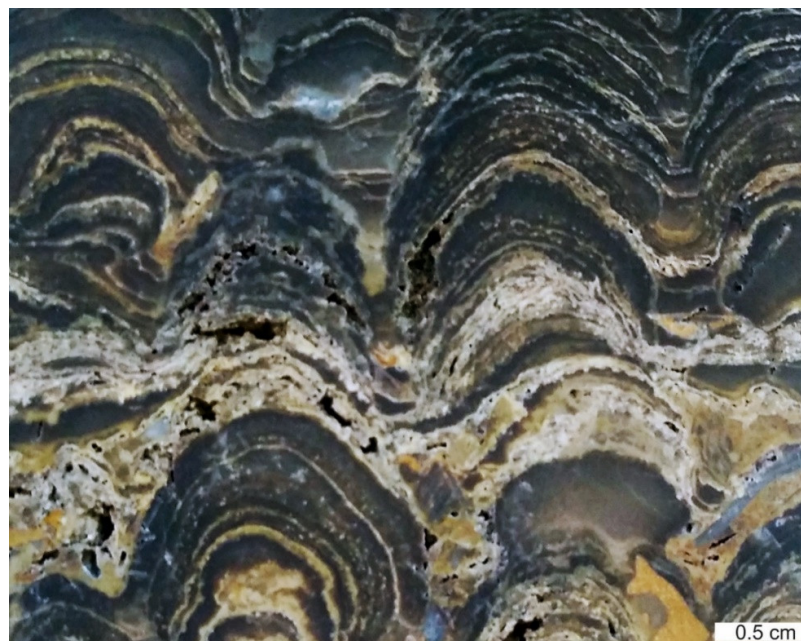
Figure 9. Overview photo of a microbe-metazoan build-up from Hardheim. The build-up is of a polished slab. It is mainly composed of columnar laminations.
