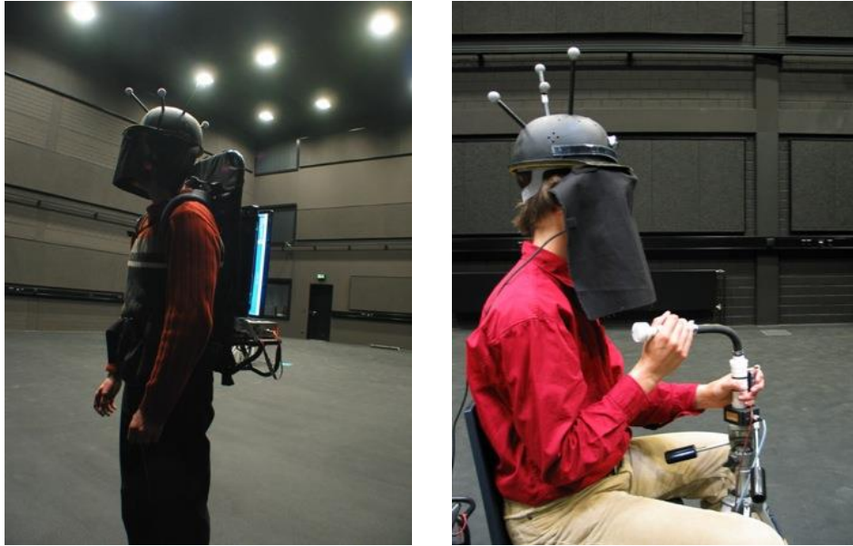
Figure 2. The virtual reality setup. The left image depicts a participant during the learning phase, equipped with a tracking helmet, a head-mounted display (HMD), and a notebook mounted on a backpack. The right image shows a participant pointing to a target during the testing phase.
