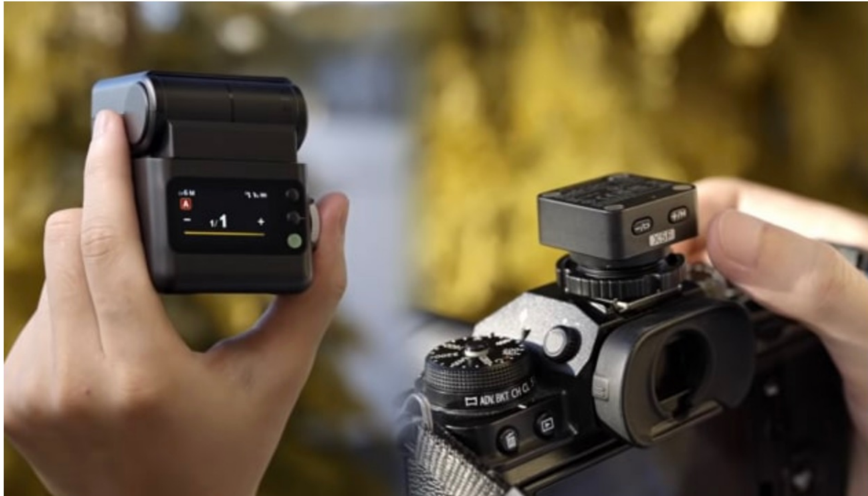
The iT32 iFlash features touch screen, rotating head and inbuilt bounce card. Image: Godox
