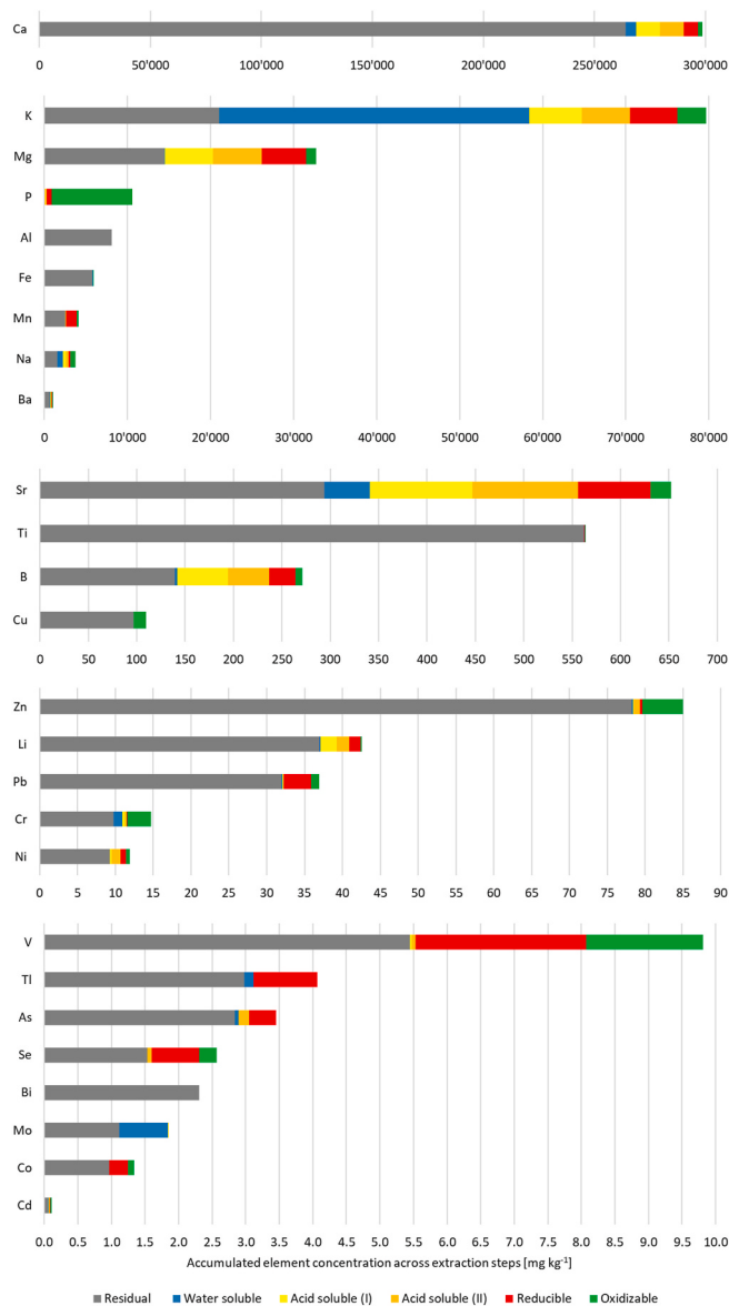
Fig. 3. Element concentration in the analyzed ash and distribution of the dissolved elements across sequential extraction steps. Dissolved concentrations [ \text{mg kg}^{-1} ] in aqueous (Water), acidic (acetic acid in two steps), reducing and oxidizing conditions. Calculated concentration remaining in the solid phase after extraction (residual fraction).
