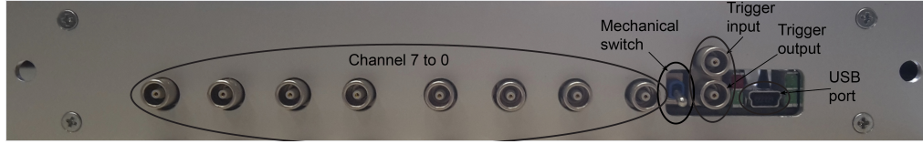
Figure 2.3: Hardware interface of the pulse generator. Beginning from the left side there are the eight output channels, the mechanical switch, the input and output channels for the trigger signals and the USB Mini-B port. The numbering of the output channels starts from the right side with zero and ends at the left side with seven.
