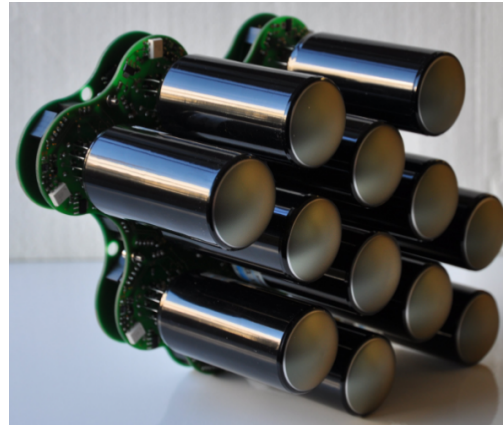
(b) A 12-pixel PMT module used in FlashCam. Credit: [62].
