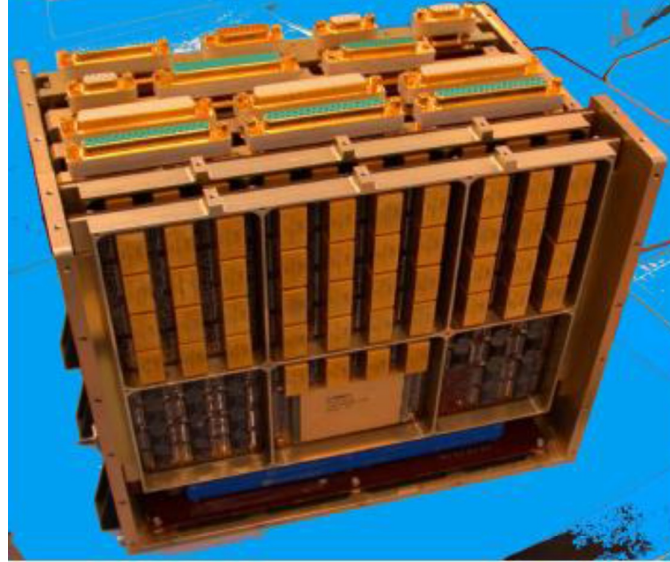
Figure 32 – The mechanical structure of one SCU with removed panels. Image: [2]
