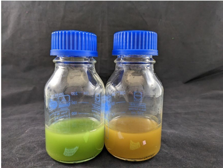
Laboratory bottles after 31 days of testing: Both bottles contain the same amount of iron. On the left, the bottle containing silicate shows a dense growth of green cyanobacteria, covering the orange iron minerals. On the right, the bottle not containing silicate shows an orange precipitation of iron minerals and less dense growth of green cyanobacteria. Photo: Carolin Dreher
