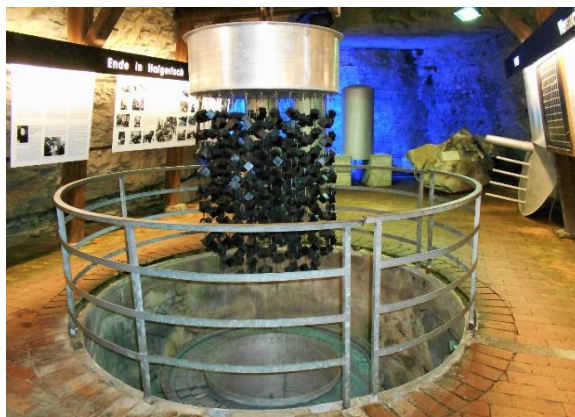
Haigerloch Atomkeller (right): Full-size replica of experimental nuclear reactor with long strings of uranium cubes.
