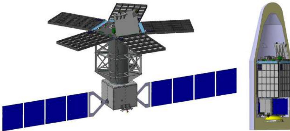
Figure 2.10: View of the LOFT Spacecraft Design concept A. The left shows the deployed configuration while the right shows the design stowed in the launcher. In this Spacecraft design there are five Panels, each containing 25 Modules. Image: LOFT Assessment Study Report
