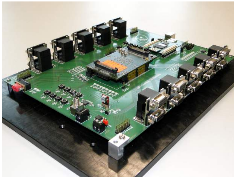
Figure 3.3: The PBEE prototype developed at IAAT. It contains an onboard MBEE simulation unit which has the ability to send 40 bit sized dummy packages. The connectors on both sides can be connected to the IAAT MBEE prototype board. This connection and the communication between the two boards has been implemented and tested in the frame of this diploma thesis. Image: Henning Wende / IAAT
