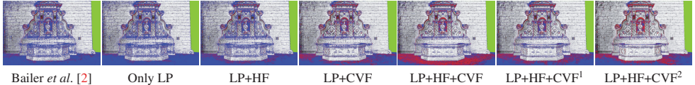
Figure 6: Relative error maps for the center view of Fountain-P11 after outlier removal, but not refined. LP+HF+CVF 1 uses cross-view filtering only for post-processing, and LP+HF+CVF 2 uses propagation-filtering at each scale without the second propagation. The blue pixels have no depth, the red have an error larger than 0.003, the green have no ground truth data, and the pixels with an error between 0 and 0.003 are marked gray 255 to 0.
