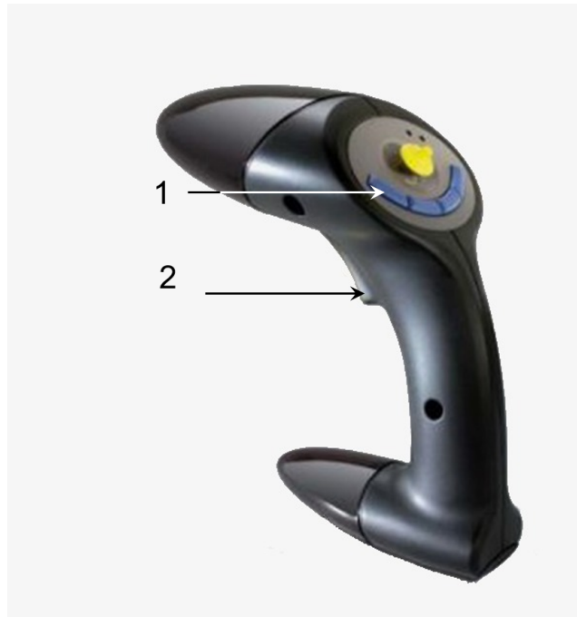
Figure 8: Flystick 2 hand held virtual reality controller to measure pointing accuracy and response time. Relevant buttons: Button 1 ( response time ) and Button 2 ( trigger ).
